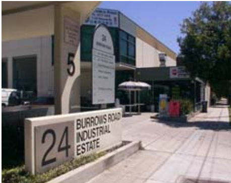
This industrial estate provides an identifiable street address and good surveillance by the placement of windows and a kiosk at the entrance to the premises.
