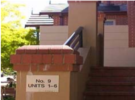
Buildings must display an identifiable street or unit number. Dwellings sharing a common entry should be restricted to between six and ten.
