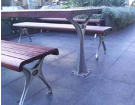
Communal or street furniture should be made of hard-wearing, vandal-resistant materials and be secured by study anchor points.
